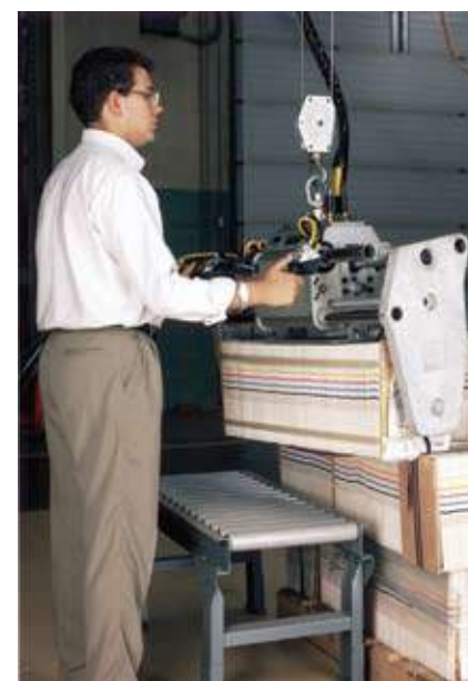
Dual cylinder with side control
