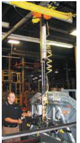
Torque tube with integrated vacuum handling device
