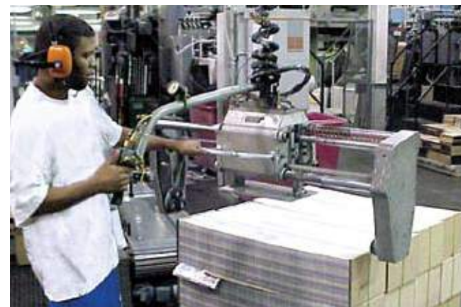
Dual cylinder with top swivel handle control
