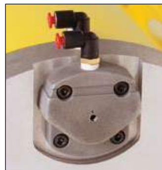
Z Stop: The optional Z Stop is a patented device that will eliminate the down-drift of suspended loads or tools during shut down or at night when the air supply is shut off. The Z Stop will stop drift within 6 inches (152.4 mm) and put the Balance Air into a mechanically locked position preventing damage to tools or objects below the suspended load. Available for use on all 10 inch (254 mm) diameter units.
